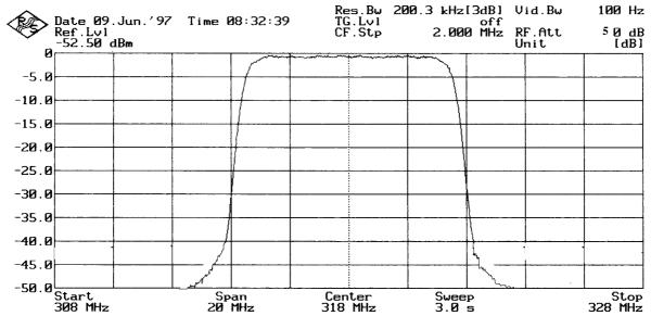
Power distribution in an 8-MHz channel with 64QAM modulation
